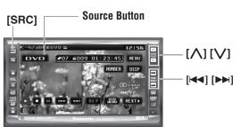
To switch Operation Screen ON, touch the center of touch panel or press [ENTER] on the remote control. (Only for Video Mode)
